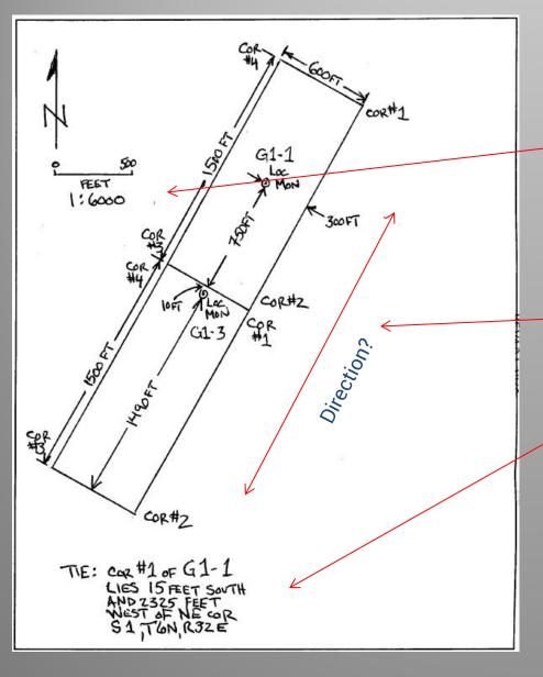
Is there a problem or mistake with the scale? Actually, no, it is accurate. In this case 1 inch = 500 feet 1:6,000 means that 1 inch = 6,000 inches or 500 ft.
